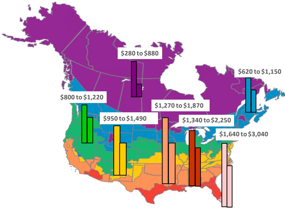
**Figure 10: Estimated Range of Net Energy Savings for a Cool Roof by Climate Zone**
