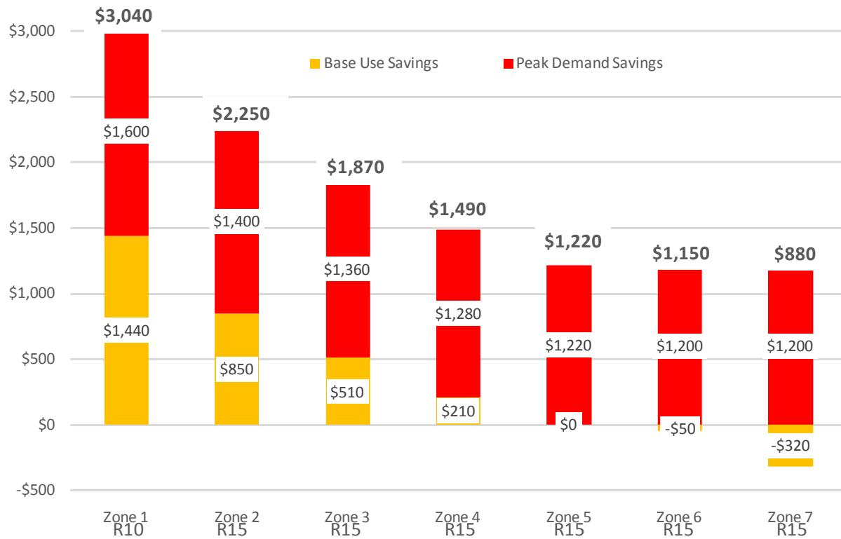
**Figure 8: Estimated Net Energy Savings: Cool Roof Installed over Existing (Old) Insulation\***
