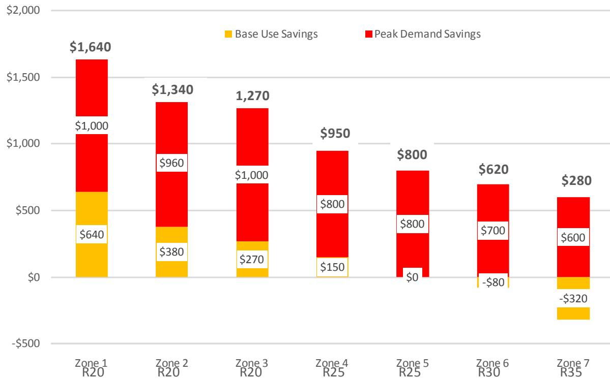
**Figure 9: Estimated Net Energy Savings: Cool Roof Installed over New Insulation**
