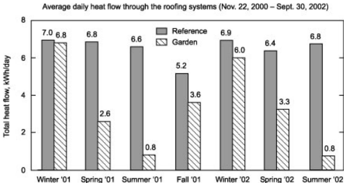
HEAT FLOW THROUGH A GREEN ROOF AND A CONVENTIONAL ROOF. THE GREEN ROOF IS PARTICULARLY EFFECTIVE AT REDUCING HEAT FLOW IN THE SPRING AND SUMMER.
